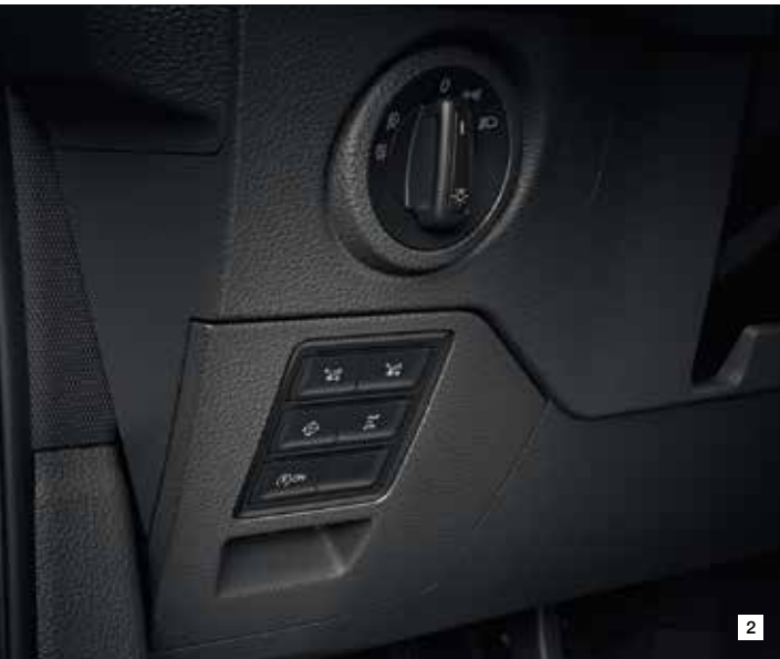
1 – Panel van Plus (available in various vehicle lengths and heights); 2 – Separate control panel for operating configurations, operable from the driver seat or outside the vehicle; 3 – Tow truck
