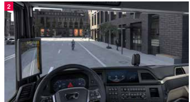
1 Front Detection 2 Emergency Brake Assist EBA Plus
