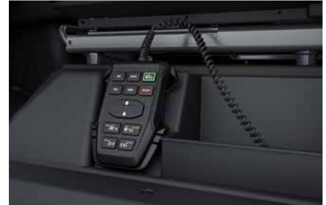
Control unit for electronically controlled air suspension (VASC)
