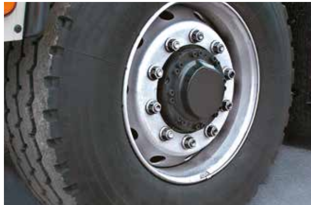
Front axle with hydrostatic wheel hub motors
